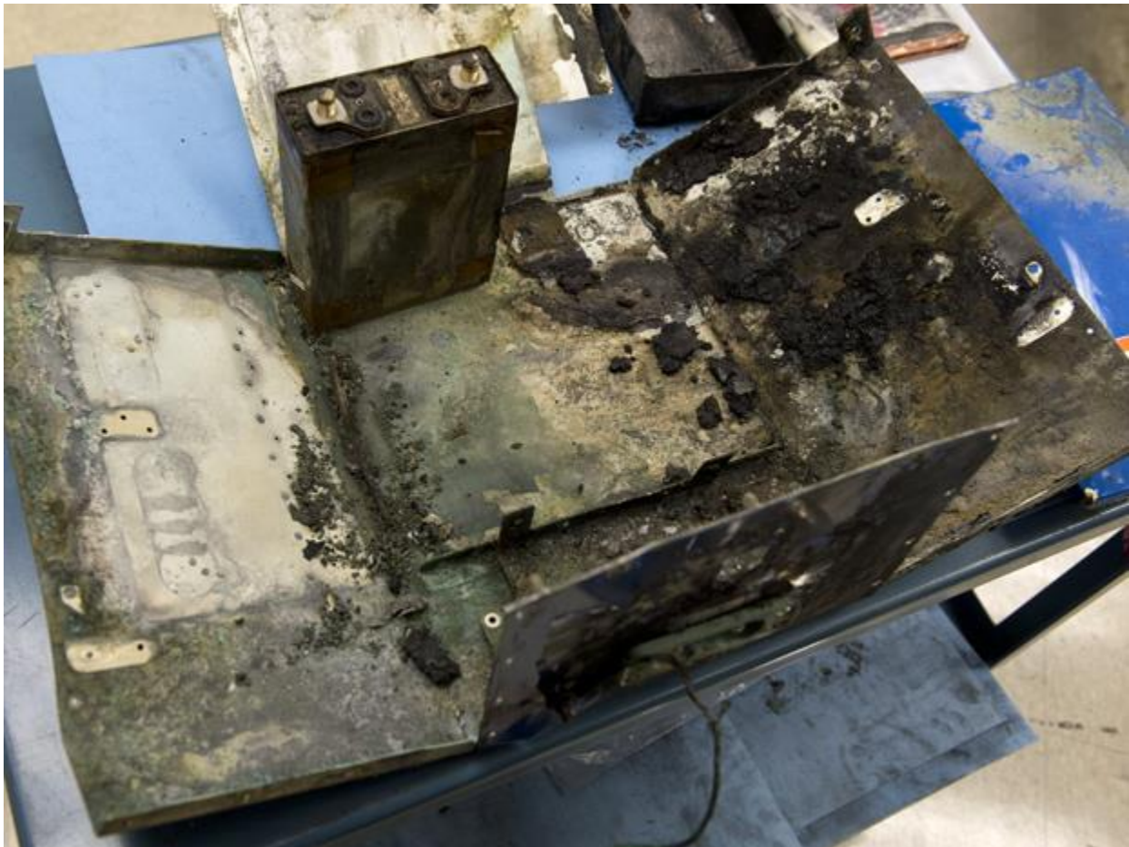
Photo: Saul Loeb/AFP/Getty Images The burned-out battery case from a Japan Airlines Boeing 787.
